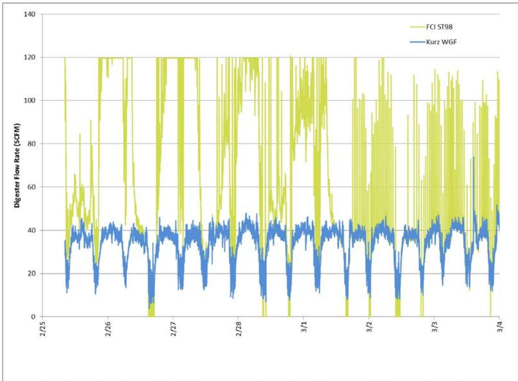
The SCADA system supports summing the data from all three digesters for 2012, when the original FCI ST98 flow meters were reporting flow. The graph clearly shows the over-reporting of gas production is related to seasonal changes in ambient temperature, with almost twice as much gas production being reported than was being consumed by the generators.
