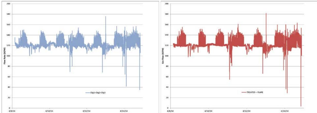
The ability to relate the long-standing discrepancy between gas measurement and actual energy recovery supported the criteria to find instrumentation capable of functioning in a condensing gas flow. Individual digester data revealed a cyclical production pattern created by our sludge doser timer setting. The ability of the Kurz WGF flow meter to show the responsiveness of digester gas to sludge feeding support the behavior we expected to see but had not been able to achieve until now.
