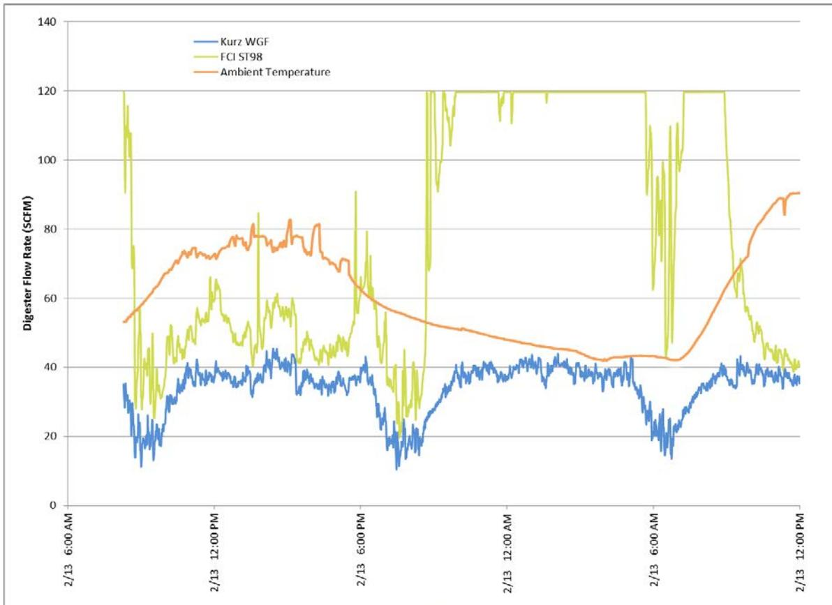
As shown in the graph, when the ambient temperature is cool (in this case, evening and early morning), the FCI ST98 flow meter reports false high readings and takes some time to respond to digester changes in cooler weather. As the outside temperatures rise, the readings from the FCI ST98 began to agree with the Kurz WGF.
