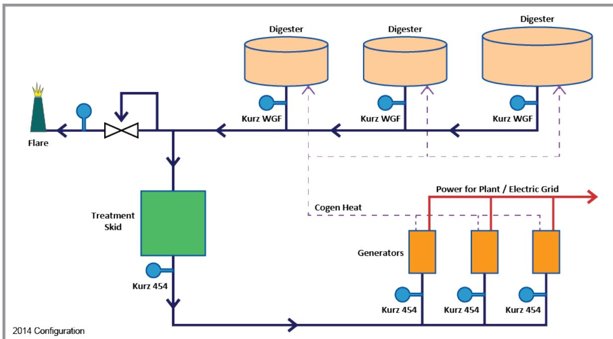
Prior to the installation of the Kurz meters biogas flow measurements remained erratic. The measurements for treated dry gas only matched overall biogas production during the heat of the day. The relationship of temperature changes, especially colder weather, affecting condensation levels and flow measurements was not fully understood at the time.
